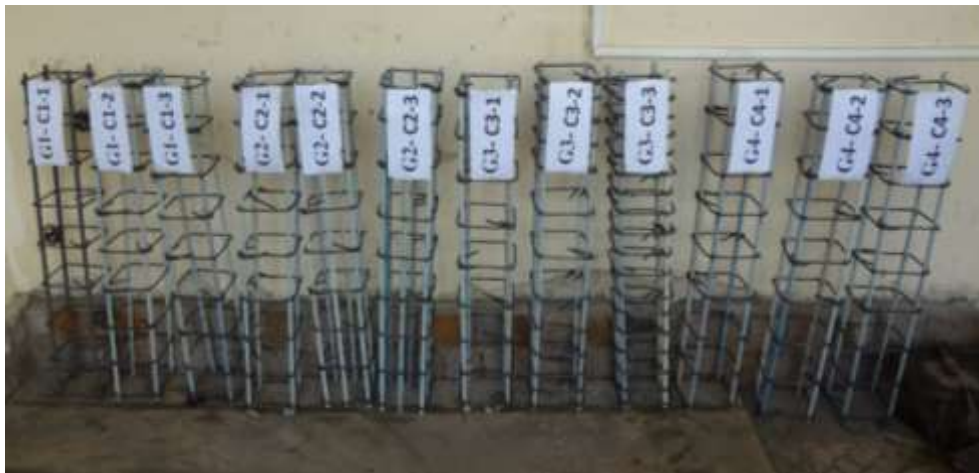
Fig. 3. Overview of the GFRP cages.
