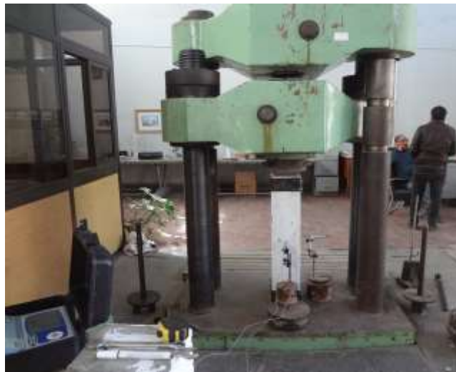
Fig. 4. Overview on setup compression tests of concrete columns.
